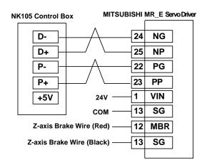
Fig. 10-7 Wiring diagram of NK105 and MITSUBISHI MR-E servo driver
