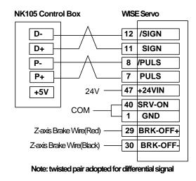
Fig. 10-2 Wiring diagram of NK105 and Wise servo driver
