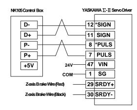
Fig. 10-3 Wiring diagram of NK105 and YASKAWA  $\Sigma\text{--}\operatorname{II}$  servo driver
