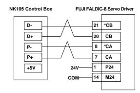
Fig. 10-8 Wiring diagram of NK105 and FUJI FALDIC- $\beta$  servo driver
